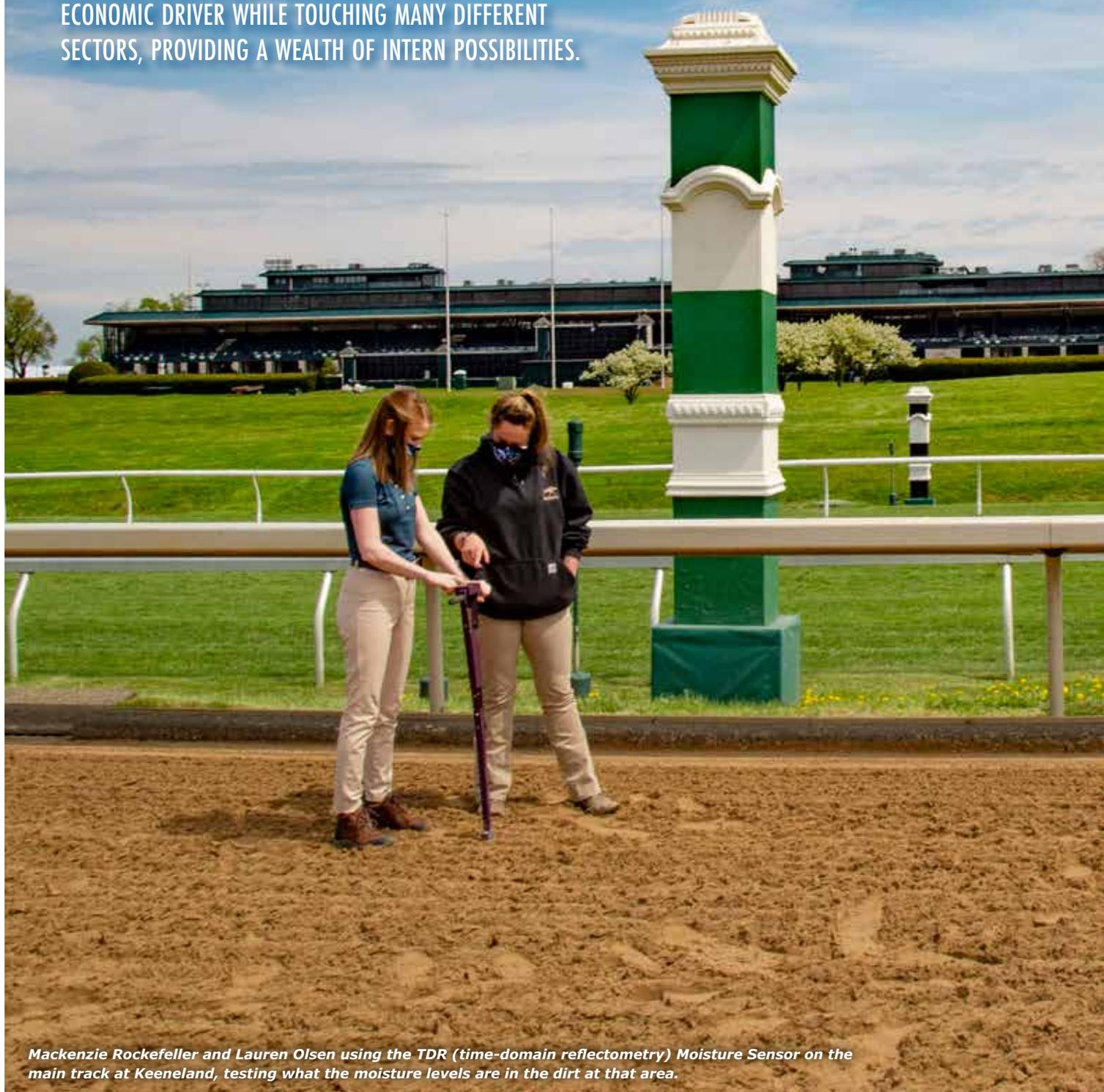
*Mackenzie Rockefeller and Lauren Olsen using the TDR (time-domain reflectometry) Moisture Sensor on the main track at Keeneland, testing what the moisture levels are in the dirt at that area.*
