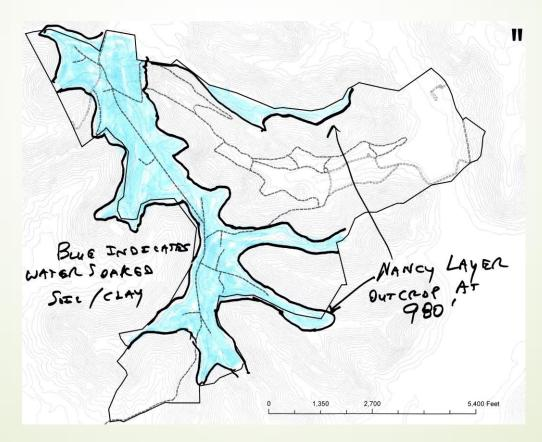
Collection System and Storage System: Pond map -112 Acre Feet capacity – 40% runoff capture
